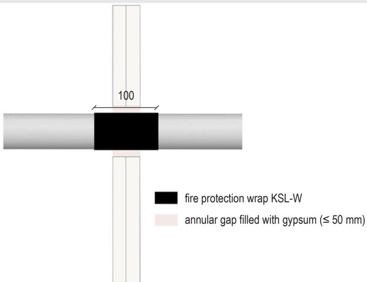
For building element and seal thicknesses see page 7. For filling the annular gap see page 11.
