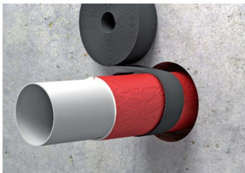
2. Glue the layers to each other by removing the protective foil. When using the non-self-adhesive variant, secure the last layer with duct tape. Then insert the wrap into the building element.
